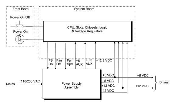
Figure 6–1. Power Distribution and Control, Block Diagram
